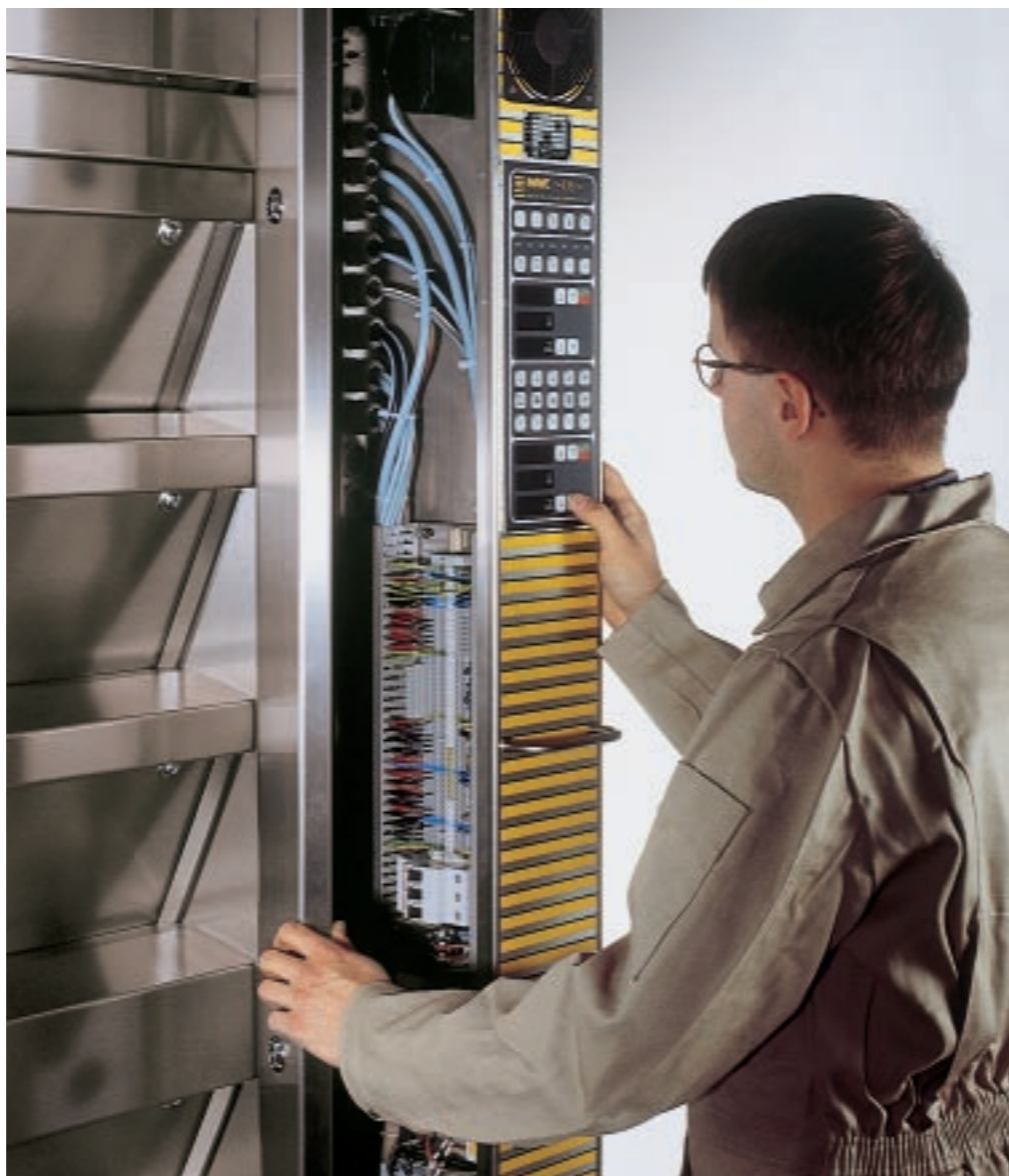
Removable oven control unit for easier maintenance
