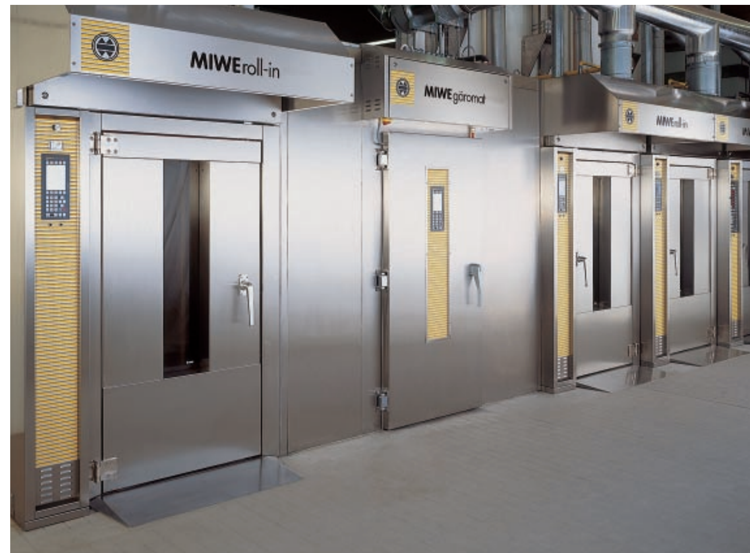
A battery of rack ovens with the MIWE gäromat proofing unit installed in between
